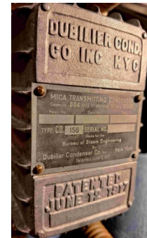
Dublier Mica Spark Transmitter "condenser" mounted on standoff insulators. Rated at .004MFD at 12,500 Volts (circa 1917)
