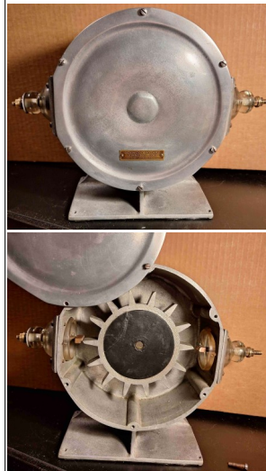
Dublier Mica Spark Transmitter "condenser" mounted on standoff insulators. Rated at .004MFD at 12,500 Volts (circa 1917)
