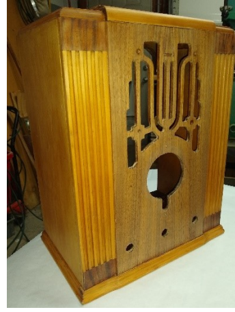
Case Sanded and Cleaned
