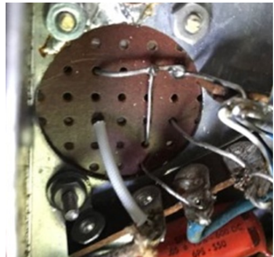
Photo 2 showing filter wired into circuitry. The inverted “L” wires connect to chassis ground
