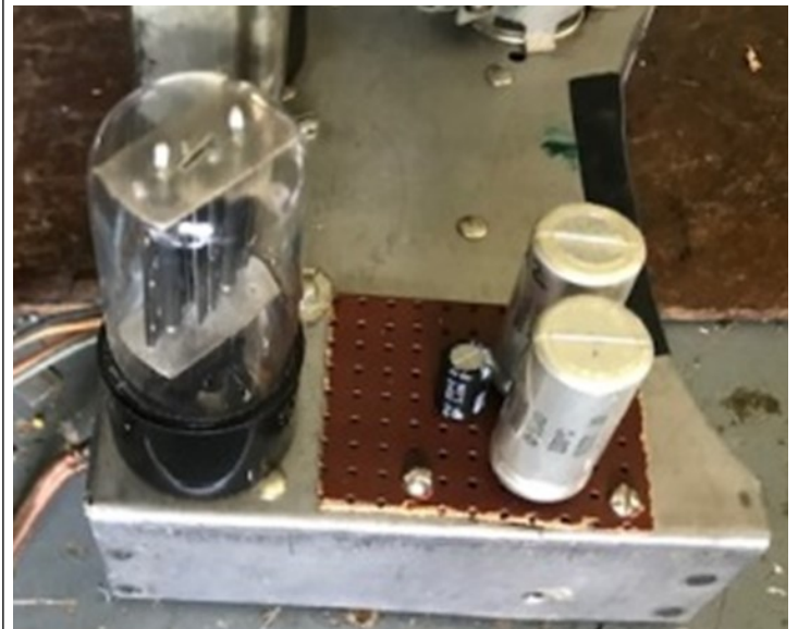
Photo 1 showing filter capacitors mounted on top of Zenith 7G605 chassis.
