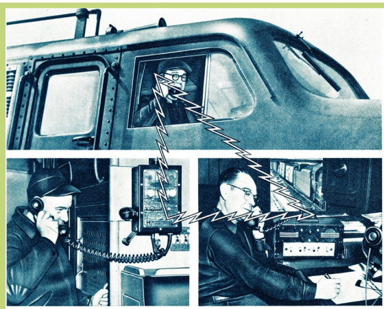
Communication en route by electronic trainphones is a modern aid to safe and efficient operation. Engineman (above) talks with conductor in the cabin car (left) and a control tower operator miles away (right).
