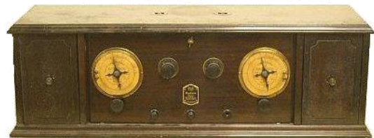
1918: Armstrong Patents the Superhetrodyne Radio. Shown: RCA Radiola AR812, the first commercial radio using the superhetrodyne circuit
