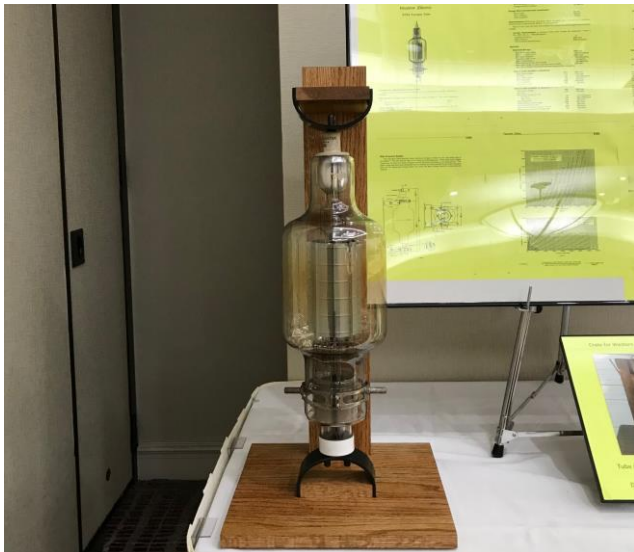
1922 Western Electric 279A Transmitting Tube
