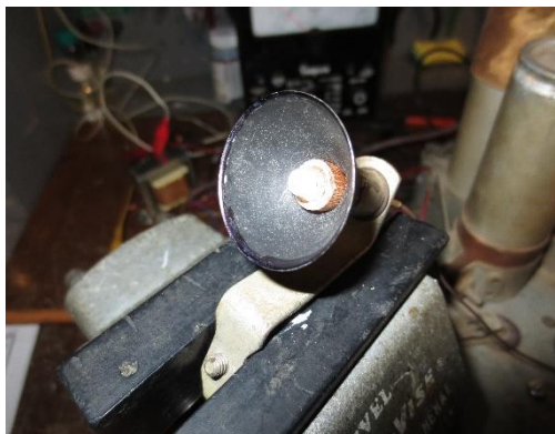
Completed LED dial lamp assembly mounted in reflector housing, powered up, and ready to install.
